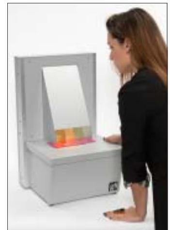
The SCV is uniquely designed to allow maximum light source selection so you can see your color under most commonly used light sources. Unit operates on 120V unless otherwise specified and uses common 24" fluorescent lamps.
